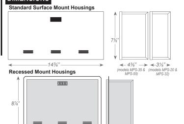
½" Extrusion from wall after installation
